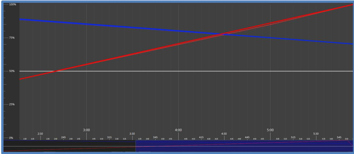
12. Adjust the level of the white light to increase from 50% at time 0:00 to 75% at time 1:00. Have the white light remain at 75% intensity for 1 hour before decreasing to 50% and holding for an hour.
