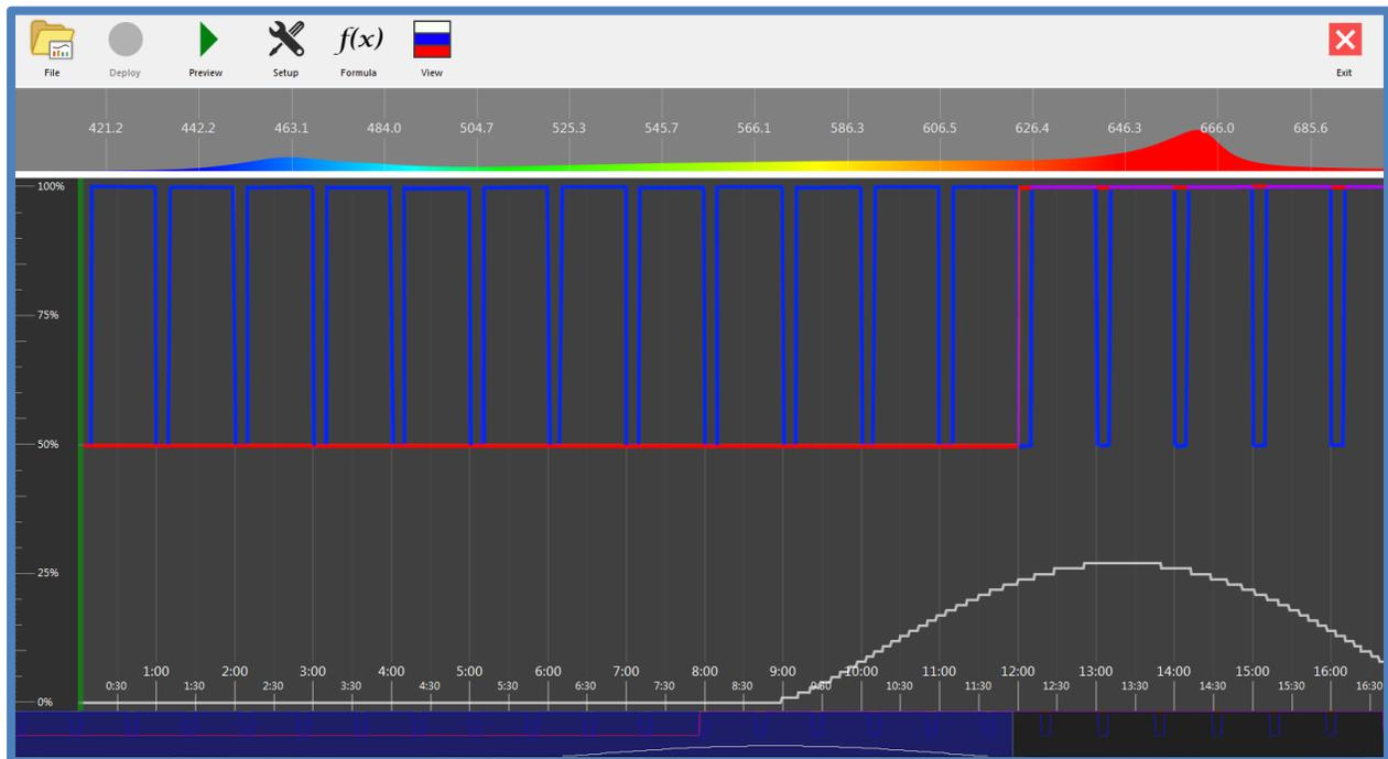
Formulas can also be combined to include multiple commands, such as “if(schedule\_hour > 12 and schedule\_minute < 10, 1, .5).” This indicates to the system that if it is more than 12 hours into the schedule, and the minute is less than 10, the light should be at 50 %. If it is later than 10 minutes into the hour, the blue will be set at 100%.
