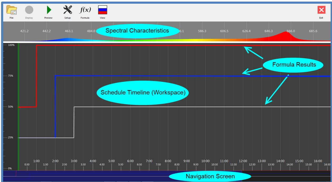
The workspace can be adjusted to include more screen-area for any of the sections. If the section visualizing the spectrum is enlarged, more information appears, such as the y-axis scale in microEinsteins.
