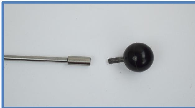
6. Replace the knob, slide the Tube Cap down the USB cable and Collapsible Slider Rod, slide the scanner into a soil or Calibration Tube and then twist the cap to secure it in place.
