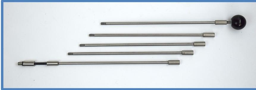
The slider rod can be used as a measuring rod, with each section of the collapsible scanner being the equivalent of the scan window length.
