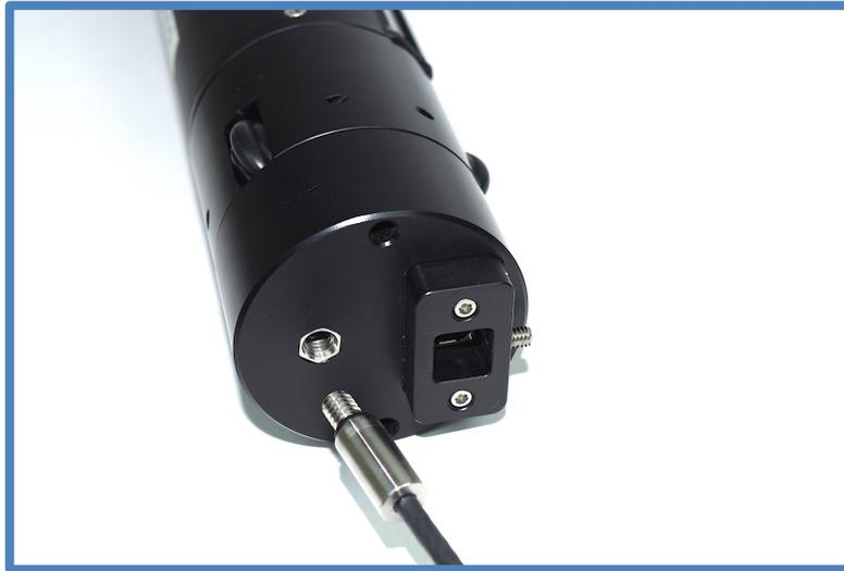
**Note:** CI-600 imaging units manufactured before March 2010 will have a U-Joint style connector instead of the more durable threaded screw connectors..
