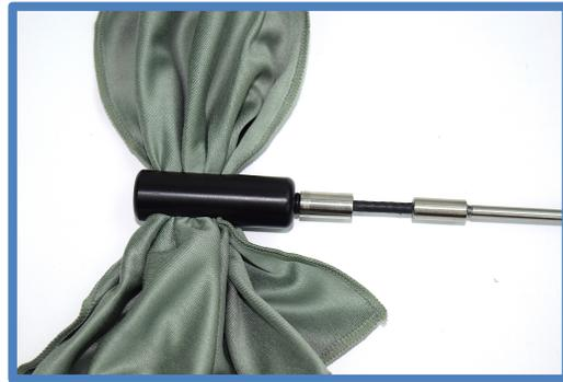
2. Lower the rod and cloth into the tube, ensuring that all sides of the tube are clean and dry.
