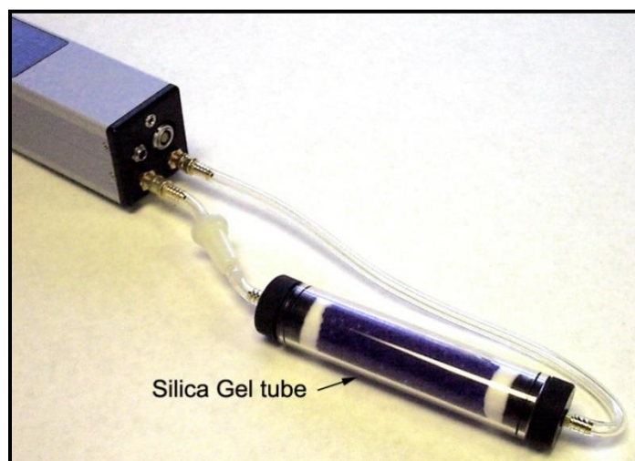
Figure 8: Configuration using Silica Gel for H 2 O calibration
