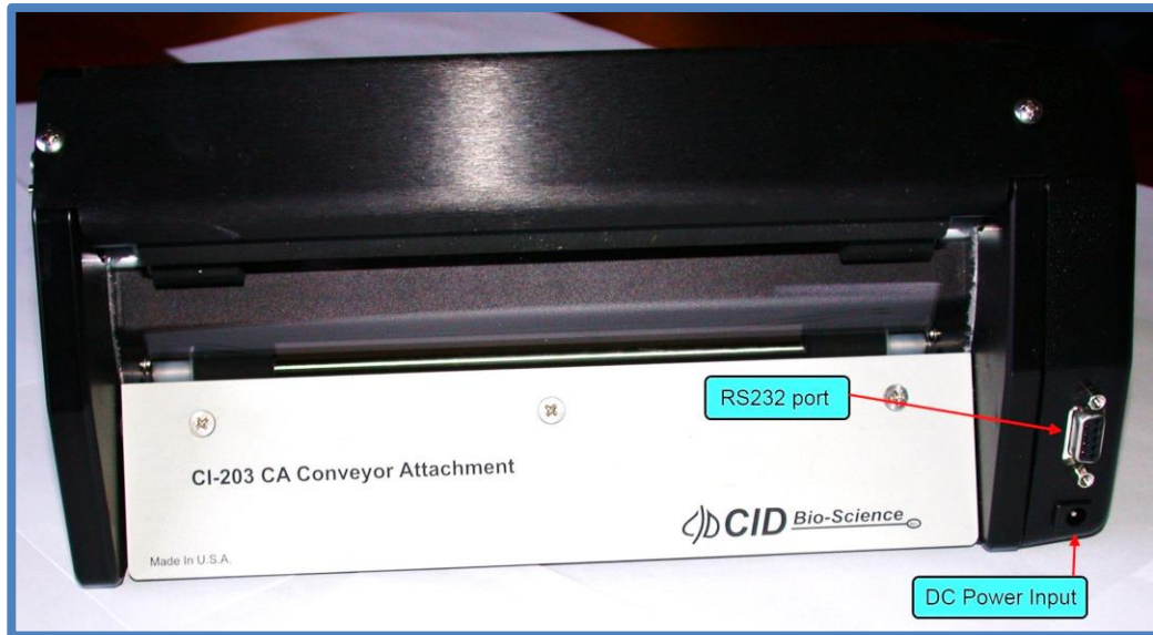
Figure 10. The RS232 port and the Power Jack of the CI-203CA.
