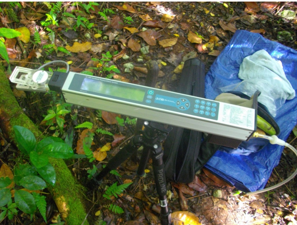
CI-340 performing “Warming Up” procedure, prior to measurements
