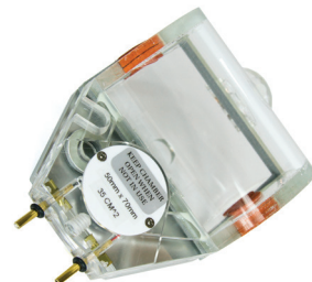
LC-5 ■ Large Cylindrical Leaf Chamber
