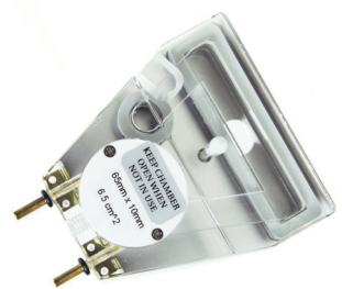
LC-3 ■ Narrow Rectangular Leaf Chamber
